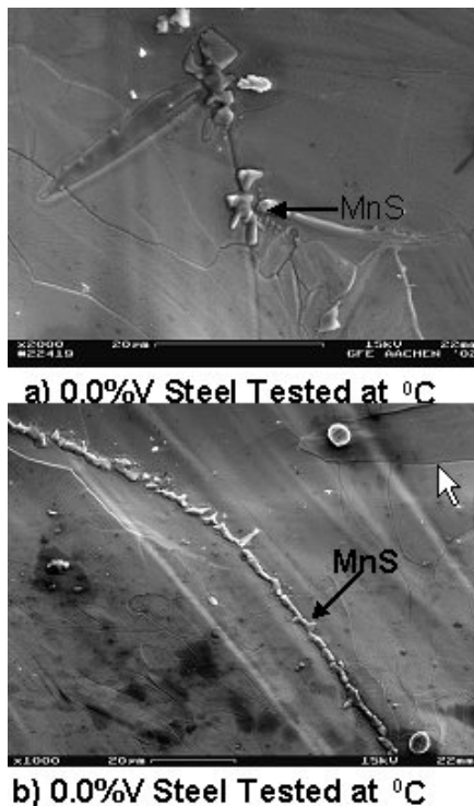
Fig. 8 Dendritic and semi-continuous MnS particles associated with low ductility.
