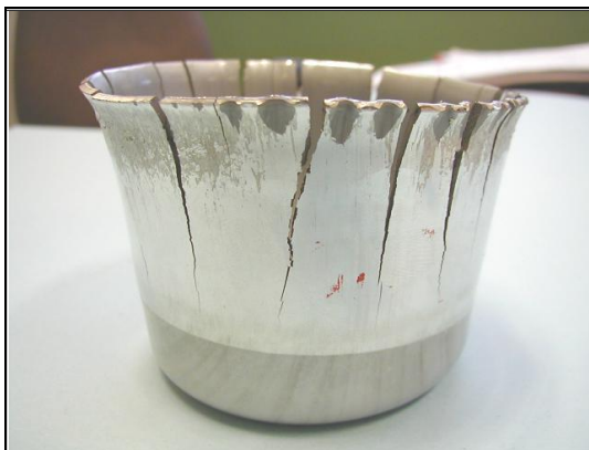
Fig.14 Hydrogen induced delayed cracking in a Fe-22Mn-0.6C fully drawn cup.
