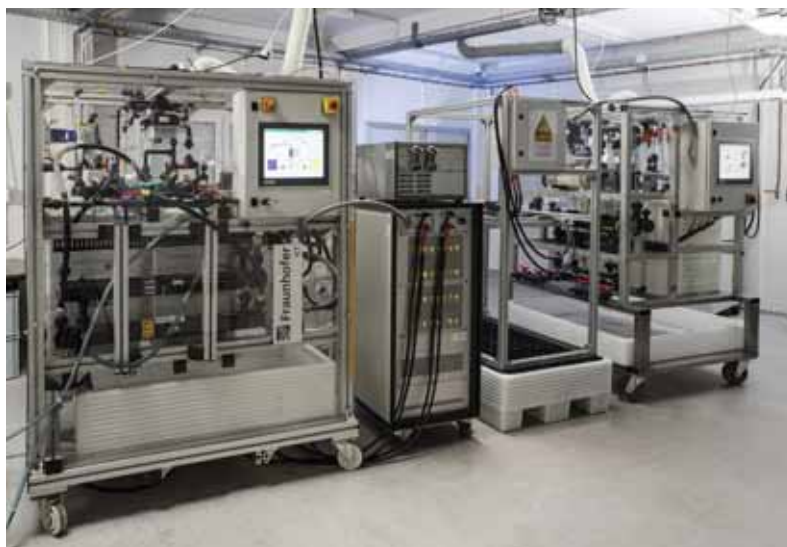
Figure 7. Two kilowatt-class vanadium redox flow battery test systems
