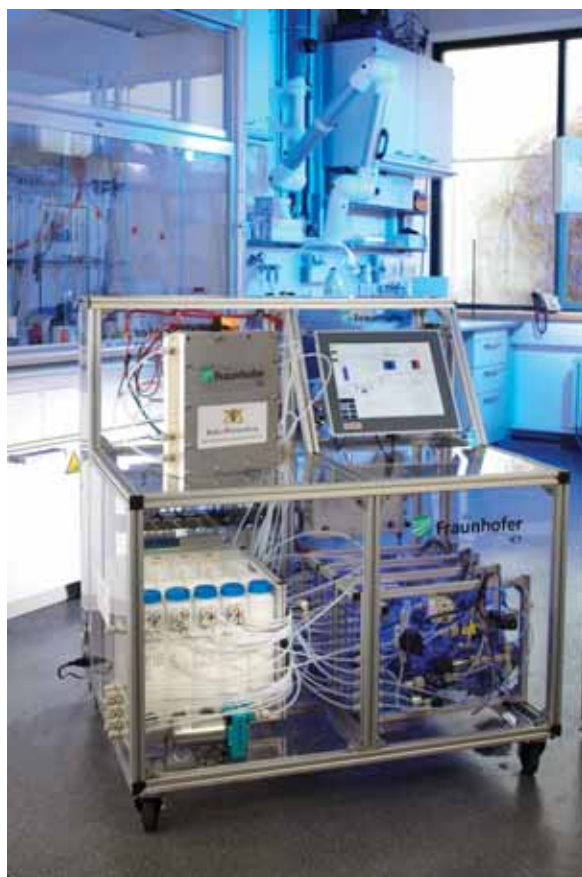
Figure 1. Kilowatt-class vanadium oxygen fuel cell system
