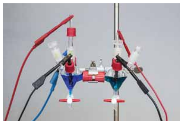
Figure 5. Discharged non-flow vanadium redox flow battery laboratory cell
