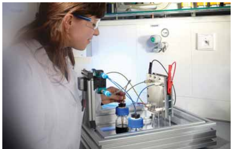
Figure 3. Vanadium redox flow laboratory test cell setup
