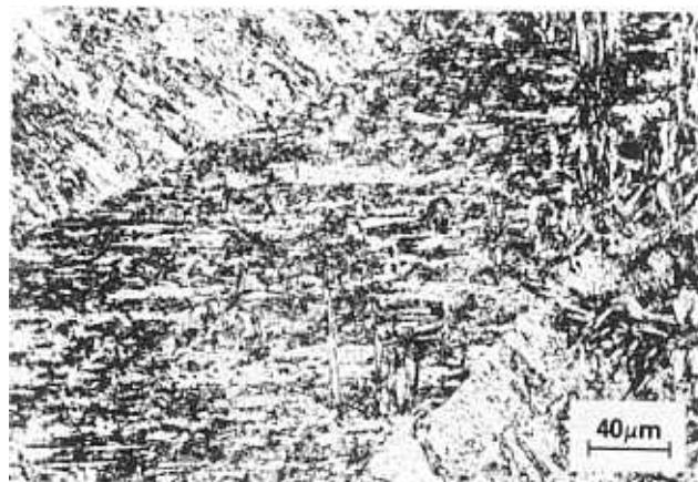
Fig. 4 Microstructure of the fusion zone of A633 Inconel 600 insert weld (Nital Etch).
