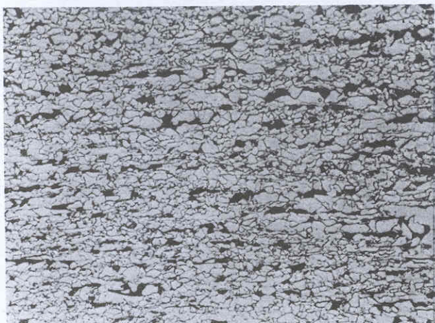
Fig. 2 - Typical microstructure of the niobium-vanadium steel (thickness 6 mm). Finishing and coiling temperature 875°C and 600°C respectively (500x).
