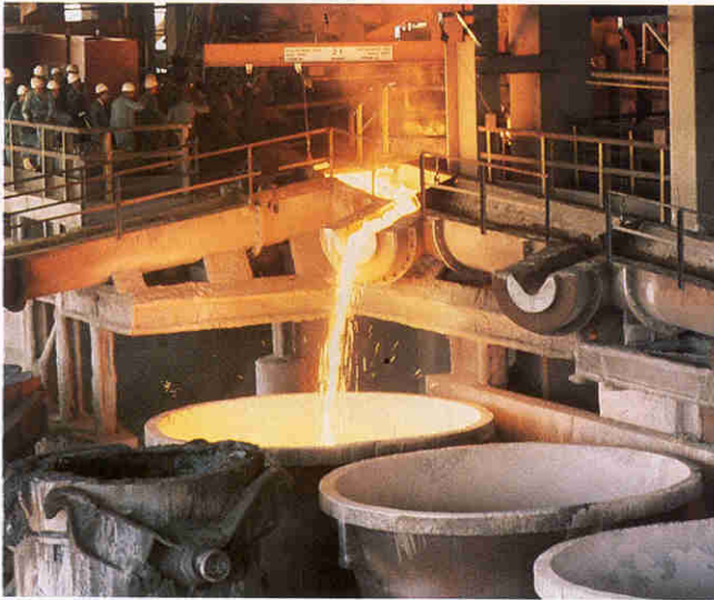
Plant for producing iron containing vanadium from titaniferous magnetite ore
