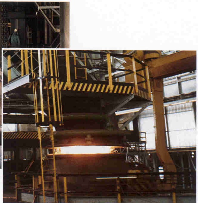
Shaking ladle producing vanadium slag from iron
