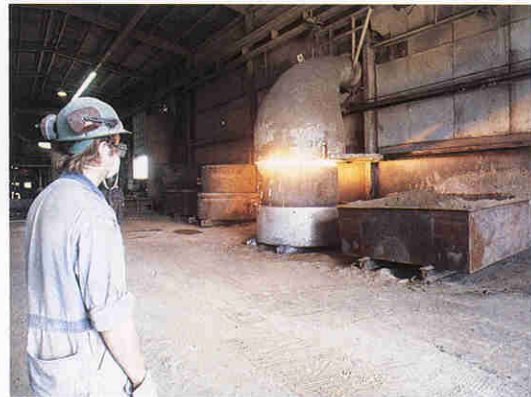
Ferro-vanadium production by the aluminothermic process.
