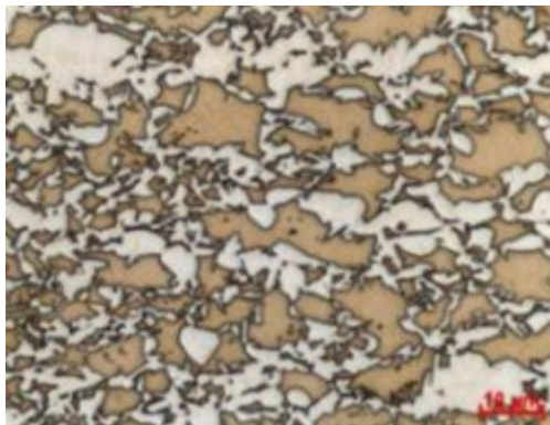
DP microstructure, martensite white, ferrite brown
