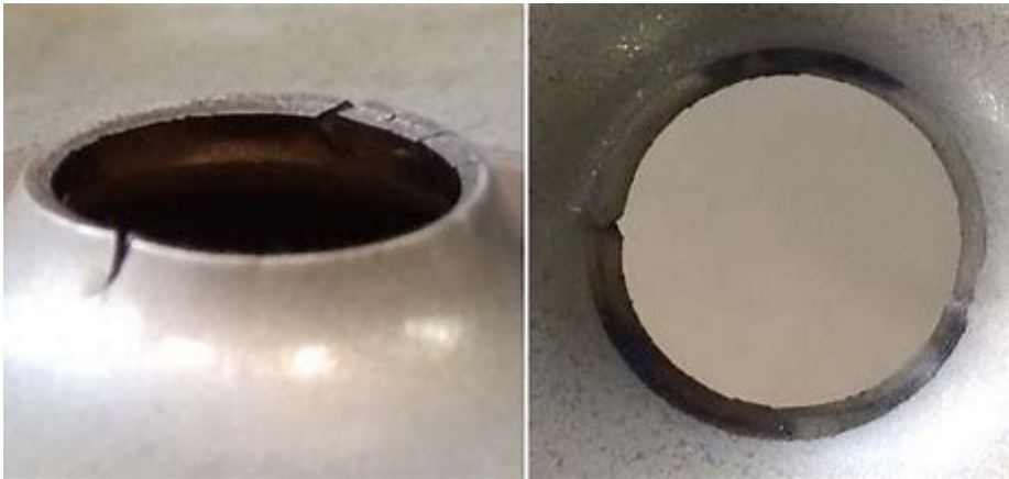
Hole expansion testing
