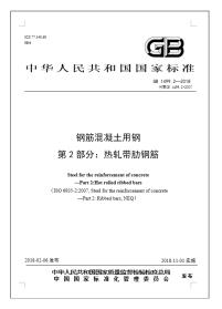
The new rebar standard, GB/T 1499.2-2018, eliminates low strength Grade 2 (335MPa) rebar and authorizes 3 different high strength standards: Grade 3 (400MPa), Grade 4 (500MPa), and Grade 5 (600MPa).
